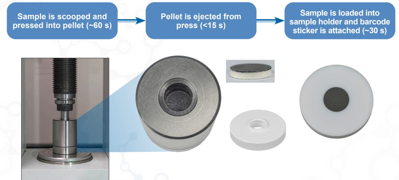
**Figure 4.** Sample preparation process is reduced from 30-60 minutes acid digestion to <2 minutes for pressed pellets.
