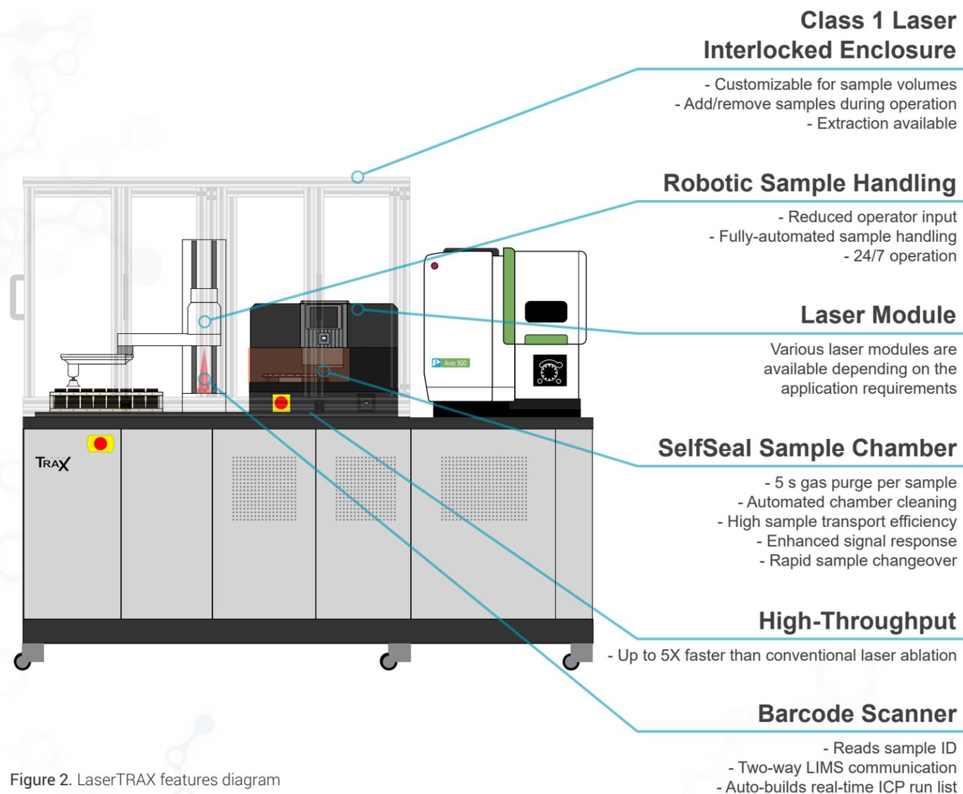
Figure 2. LaserTRAX features diagram
